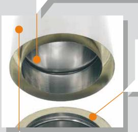
Intermediate layer acts as insulation, made up of high density (110 kg/m3) radiating basaltic rock wool with 25/50 mm thickness and 0.058W/ mK conductivity (at 200°C temperature).
